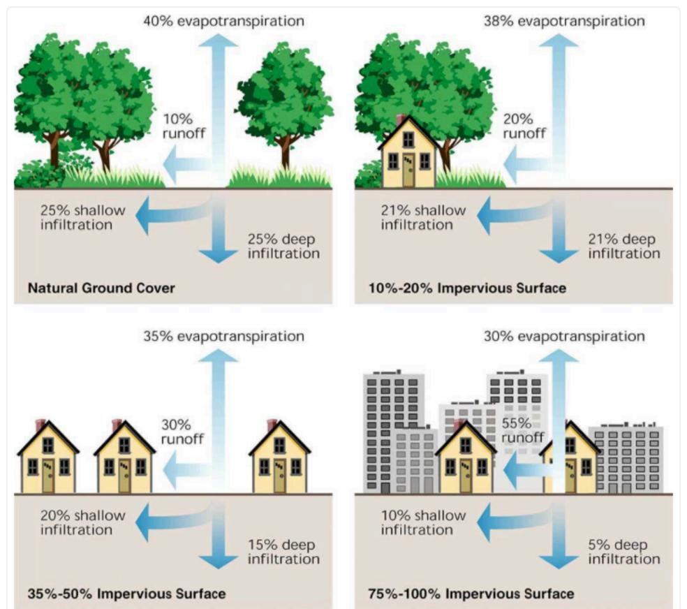
For natural ground cover, only 10% of rainfall runs off. The runoff percentage increases as imperviousness increases. For land that is 75-100% impervious, 55% of rainfall runs off.
